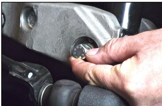
7. Lock the screw securing the bottom of the side sleeve to the parallelogram at a torque of **45 ÷ 50 Nm**;
