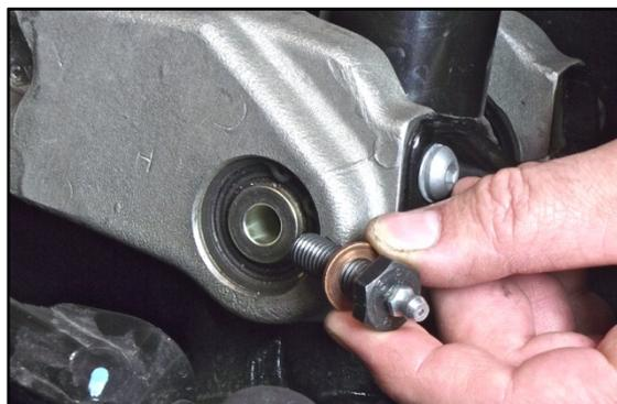
3. Lock the special tool at a torque of  $14 \div 20$  Nm;
