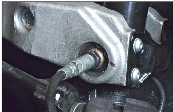
5. Pump the grease into the housing of the bearing until detecting leakage from the sealing surface of the lower dust gaiter;
