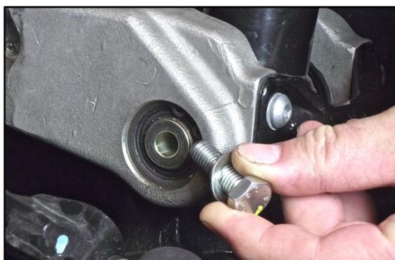
2. Install the special tool with the copper washer;
