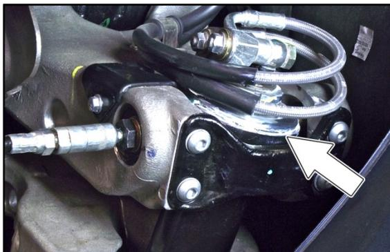
9. Lock the screw securing the top of the side sleeve to the parallelogram at a torque of **45 ÷ 50 Nm**.
